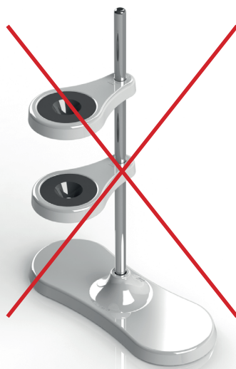
Wrong position of the funnel holders -Danger of tipping over!
